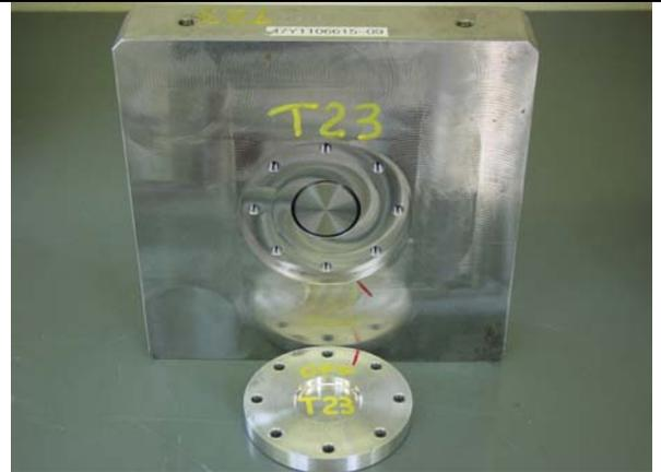
**Figure 6. View of the rear of a Be target with the rear aluminum plate removed, showing the back side of the Be disk.**
