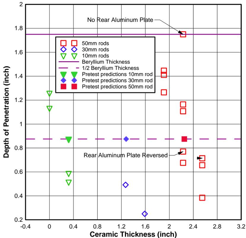
**Figure 13. Results of the experiments with beryllium targets. Note the solid figures that indicate the pre-test analytic model predictions.**
