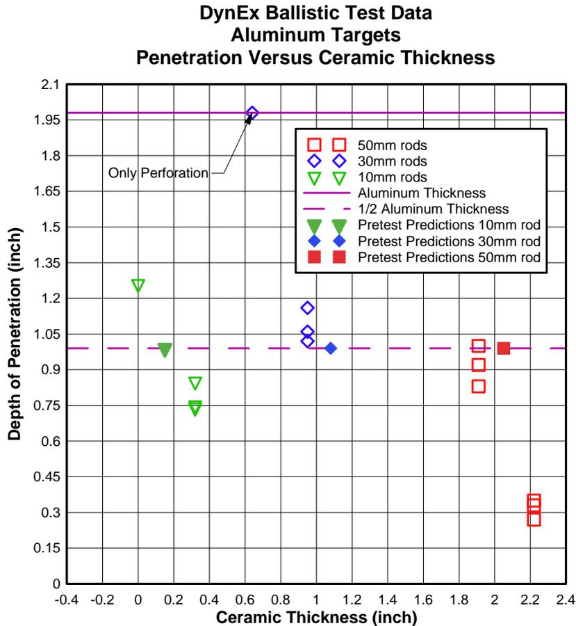
**Figure 12. Results of the experiments with aluminum targets. Note the solid figures that indicate the pre-test analytic model predictions.**
