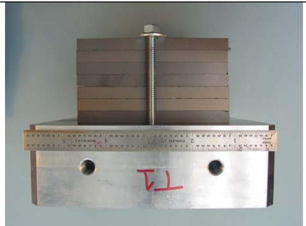
Figure 4. Top view of an Al target, showing the stack of B4C armor disks before impact (Test 1).
