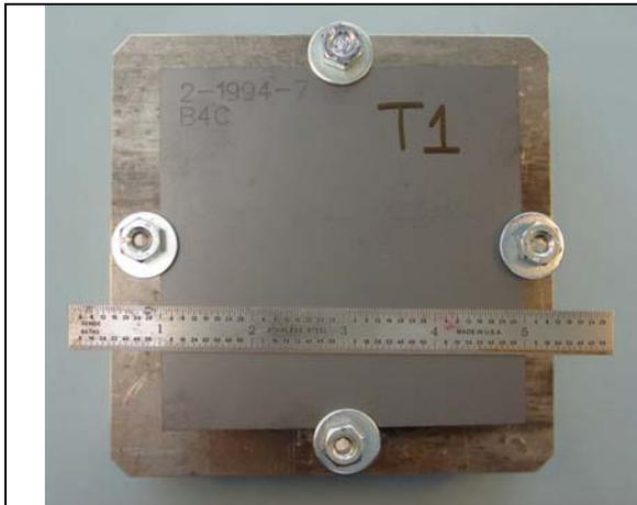
Figure 3. Impact side of the Al target, showing the B4C ceramic armor disks.
