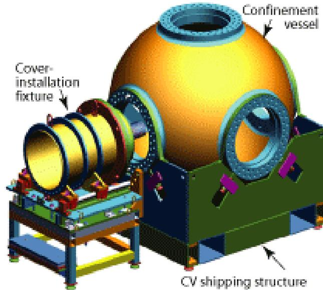
**Figure 1. A DynEx containment vessel configuration.**
