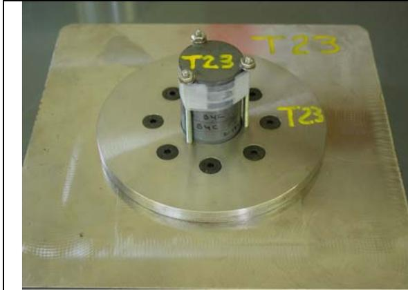
**Figure 5. View of the front of a Be target showing the stack of B4C armor tiles (above the impact side of the Be piece).**
