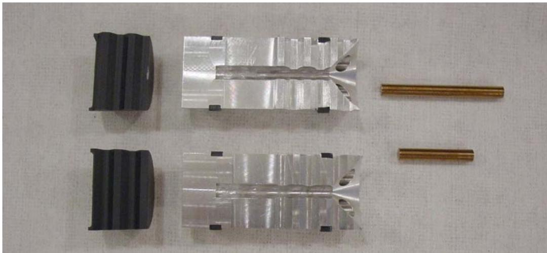
**Figure 7. Photo of the 2-piece sabot and the 50mm and 30mm length rods.**
