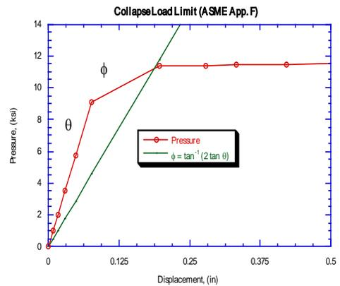
Figure 7. Collapse Load Limit (per ASME Section III, Division 1, Appendix F)
