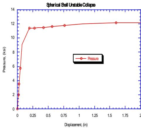
Figure 6. Spherical Shell Static Load-Deflection Curve
