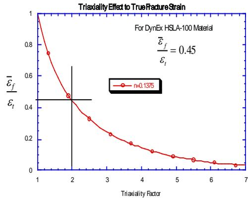
Figure 14. Triaxiality Factor For HSLA-100 Spherical Vessels
