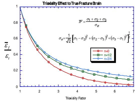
Figure 13. Triaxiality Effect On True Fracture Strain
