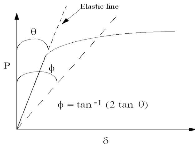
**Figure 3. Load-Deflection Characteristic For Static Collapse**
