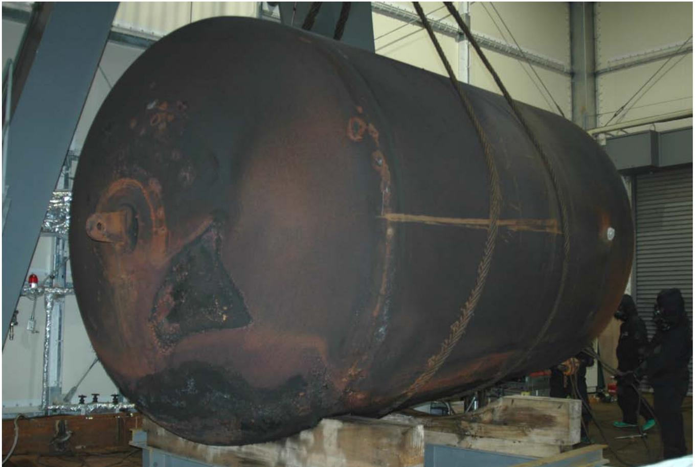
**Figure 4.** External surface of DAVINCH inner vessel after removal from the outer vessel.
