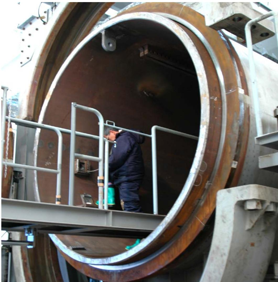
**Figure 3.** View of DAVINCH with top heads of both the inner and outer vessels removed.
