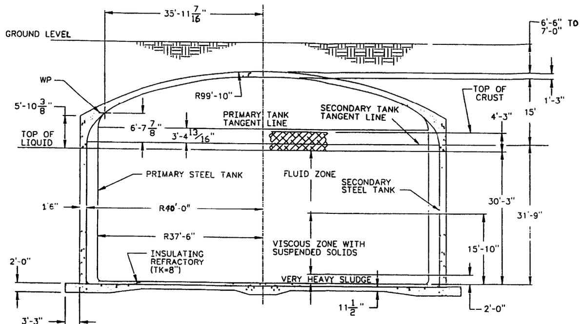
Fig. 2. Tank 101-SY cross-sectional dimensions.
