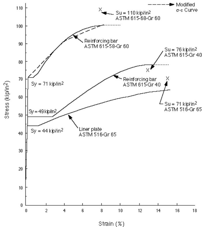
Fig. 5. Engineering stress-strain relationship of American Society for Testing and Materials (ASTM) steels.
