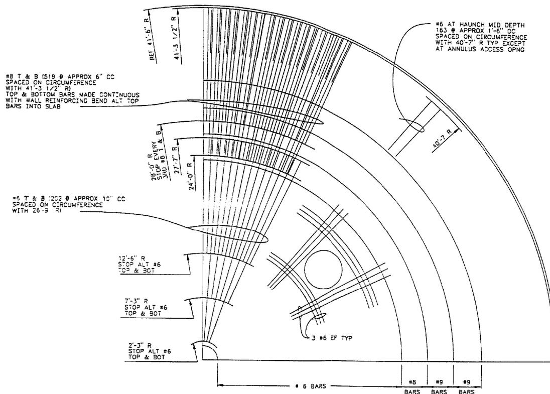
Fig. 6. Dome reinforcing-bar details.
