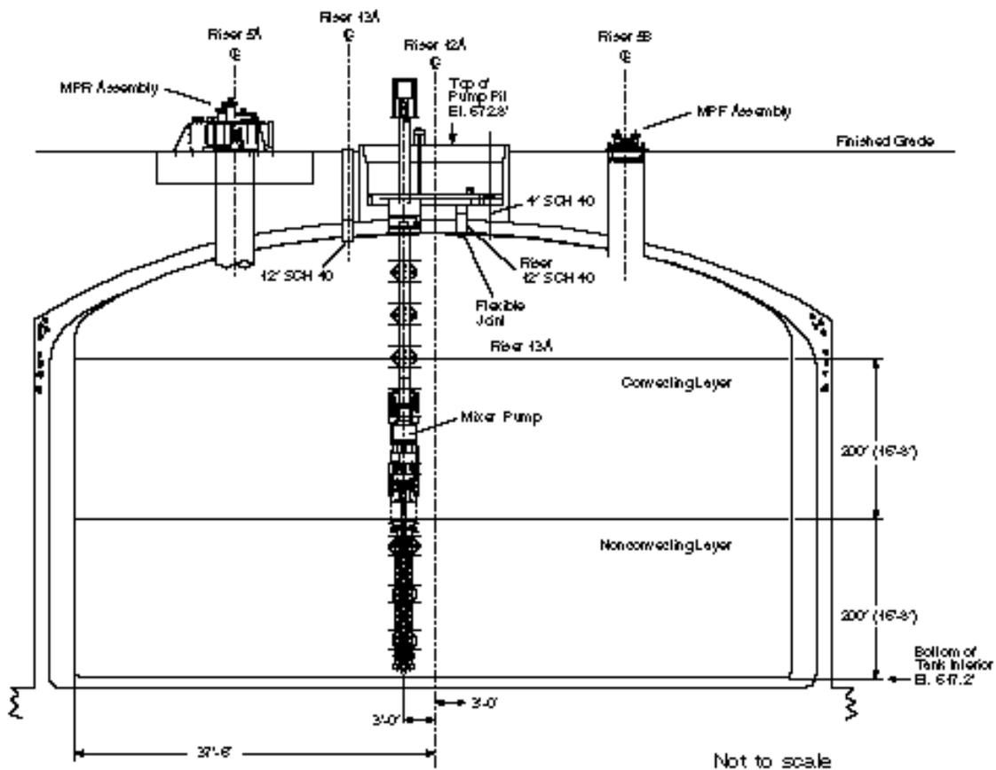
Fig. 1. Cross-sectional view of Tank 241-SY-101.
