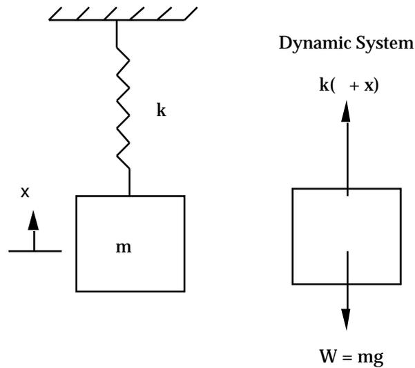
Fig. 3. Simple SDOF oscillator.
