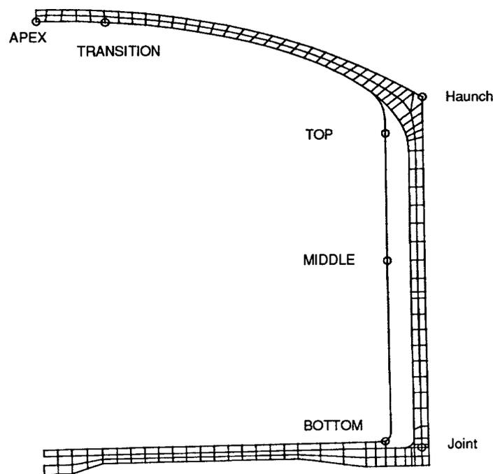
Fig. 4. Axisymmetric FEM of Tank 101-SY.
